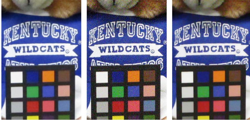
Figure 3.2: JPEG Crops from Canon A4000 at ISO 1600, 16x ISO 100, and 16x ISO 100 Filtered
